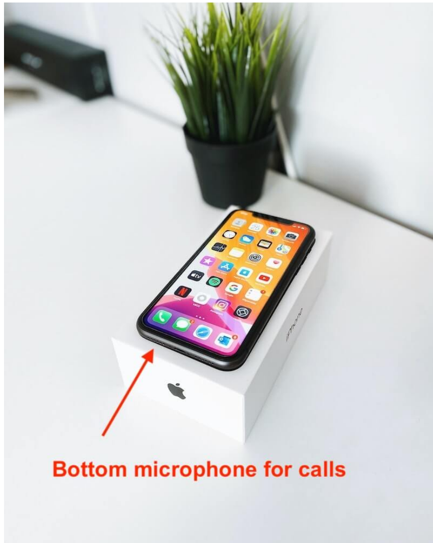
Figure 21: Bottom MEMS Microphone Location [38]
