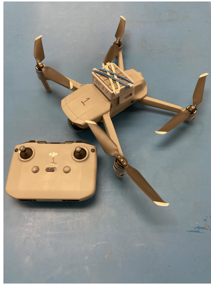
Figure 34: Drone Mounted With Payload Basket
