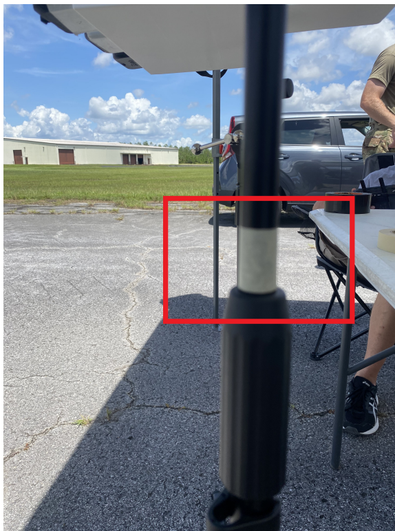
Figure 32: Tape Used To Set 1 m Height
