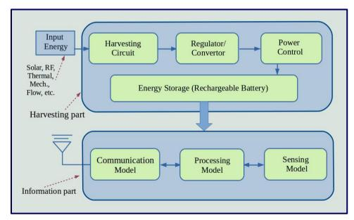
Fig. 4 - A general architecture of the energy-harvesting node
