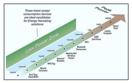
Fig. 5 - Peak Power Levels for Typical IoT Devices (Source: [55])
