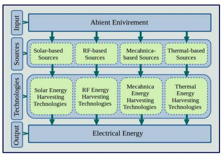
Fig. 3 - Ambient energy-harvesting sources for IoT-based wireless nodes
