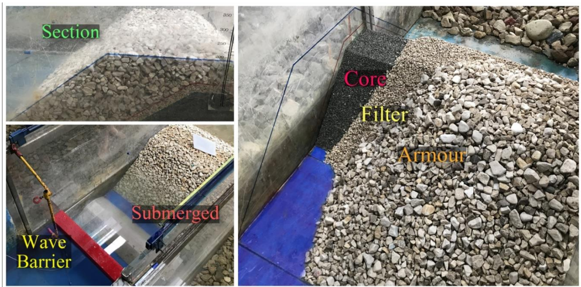
Fig. 4 - Images of RMB layers, submerged obstacle, and floating wave barrier
