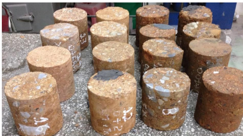
Fig. 4 - Series of extracted specimens used for the experimental assessment
