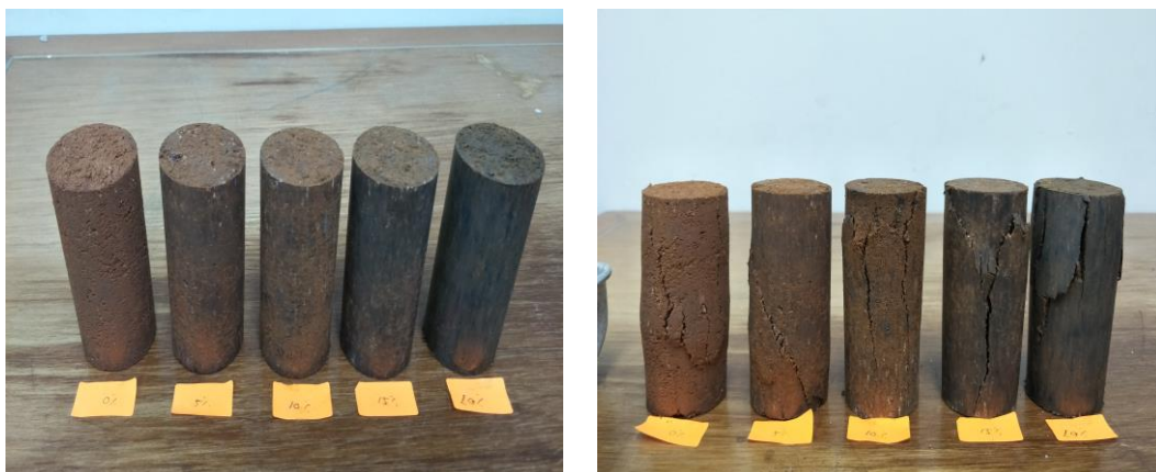
Fig. 5 - (a) Sample before UCT; (b) Sample after UCT
