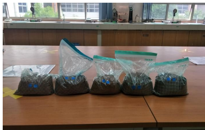
Fig. 1 - Sample at different percentage of geopolymer
