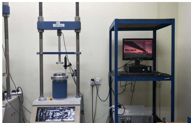
Fig. 3 - Unconfined compressive strength machine
