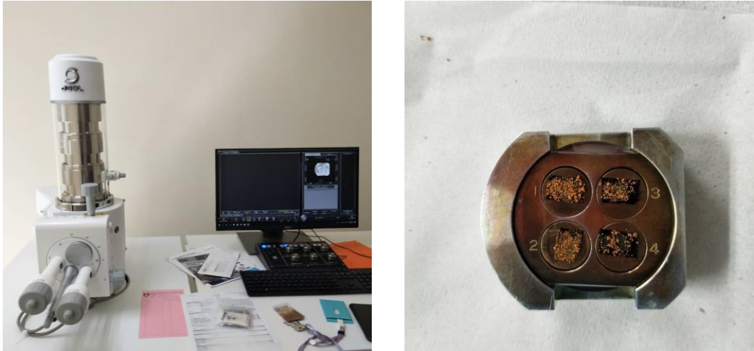
Fig. 4 - (a) SEM Machine; (b) SEM Sample Preparation
