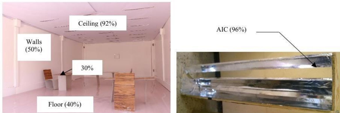
Fig. 6 - (a) Interior photometric properties; (b) Exterior anidolic element reflectance
