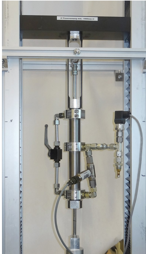
Illustration 4.7: Single Friction Point Test Rig (2) – overall setup
