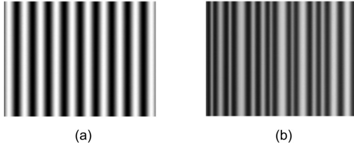
Fig. 4.3 Example of (a) sinusoidal periodic fringes and (b) sinusoidal aperiodic fringes.
