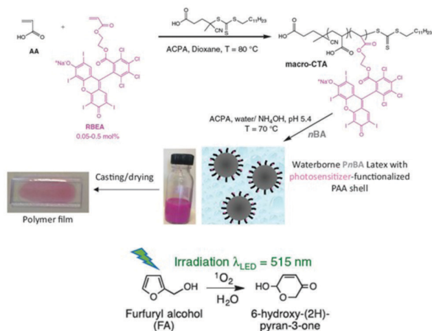
Fig. 12 Schematic illustration for the synthesis of photoactive latex particles and films. 218 Reprinted with permission from ref. 218. © 2018 Wiley-VCH Verlag GmbH & Co.
