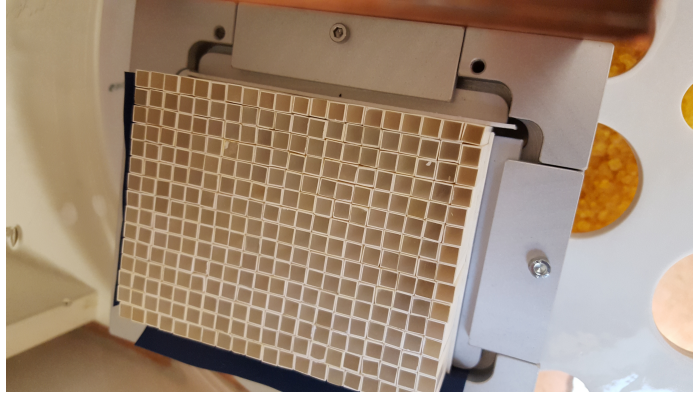
Figure 3.26.: A photograph of the 15 by 20 CsI(Tl) crystal matrix used in the SPD. The individual crystals are unique and have reflective titanium dioxide coatings of varying thickness to avoid optical crosstalk, which makes them appear to have different levels of opacity.
