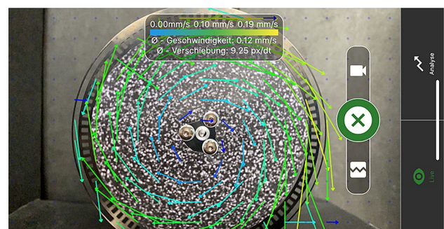
Fig. 1 Main menu of the SmartPIV app showing the option data evaluation, recording and live preview (here cross-correlation analysis of a rotating disk)
