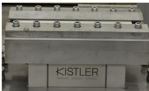
Fig. 5 Clamping technique with multi-component dynamometer for process force measurement
