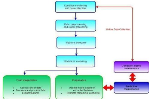
Fig. 7: Maintenance for Data Center Operation Management
