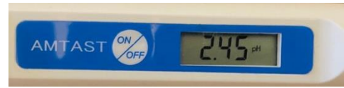
Figure 3: pH measurement on AMT28F pH meter (Actual reading for lemon fruit, with exposure, Time interval of 10 seconds)
