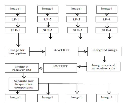
Fig. 03: Proposed Multiple Image Encryption technique based on 4-WFRFT.
