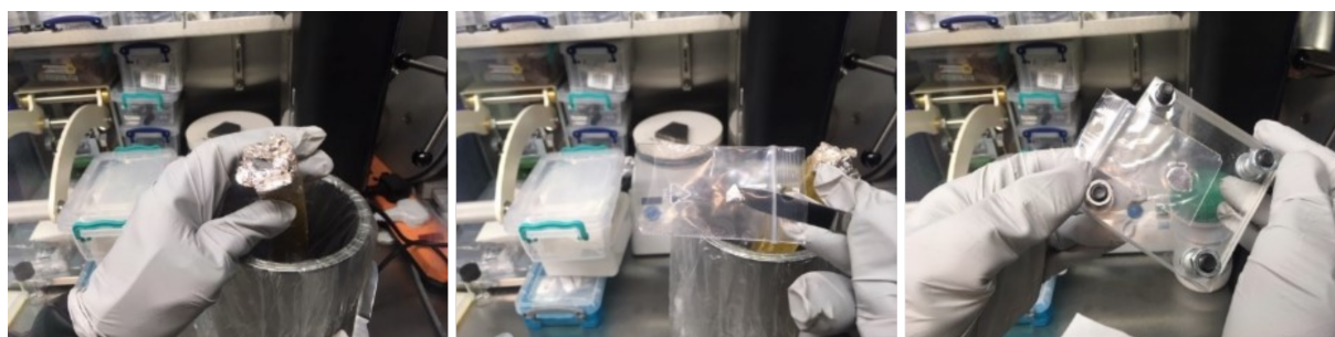
Figure 4.12: Na metal electrodes preparation. (left) a piece of \text{Na}^0 is cut from a rod; (center) the piece is placed in a LDPE; (right) the piece is pressed into a foil. Circular electrodes are then punched from the foil (not illustrated here).
