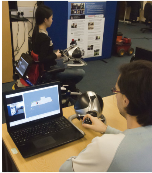
Figure 2.1: Example of LAD being used in a smart wheelchair application. The driver attempts to navigate a difficult scene while being observed by the assistant, which provides a helping control signal as needed. The interaction is recorded and then used to train a model. If learning is successful, the model should be able to autonomously replicate the demonstrated assistive behaviour. Excerpt from (Kucukyilmaz and Demiris 2015).
