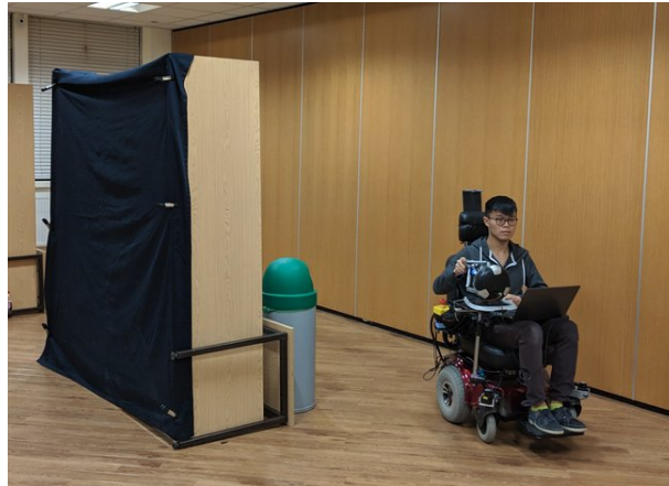
Figure 3.10: Shows a user driving in obstacle course while data is recorded. The driver was impaired by a simulated disability, which used the force-feedback joystick to impose a tremor on their hand. Two users participated in the data collection, being tasked with repeatedly reaching pre-defined goal locations.
