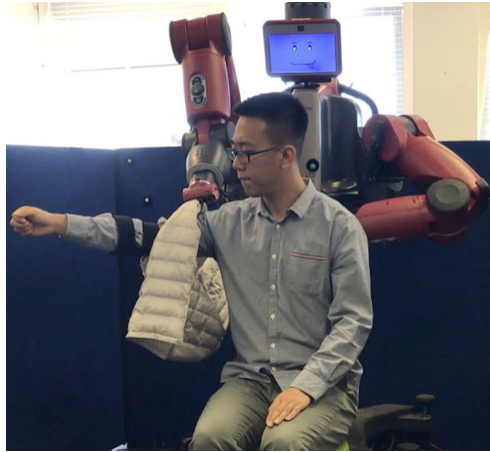
Figure 1.1: Example of an assistive robotics application, where a robot helps a person with reduced mobility get dressed. Excerpt from (Zhang, Cully, and Demiris 2019)
