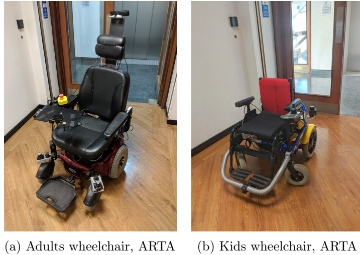
Figure 3.2: Different smart wheelchairs that can be used with our teleoperation platform. Despite being different from physical and electronic points of view, a wrapping software layer is used to guarantee that, from a high-level perspective, the wheelchairs can be used interchangeably.
