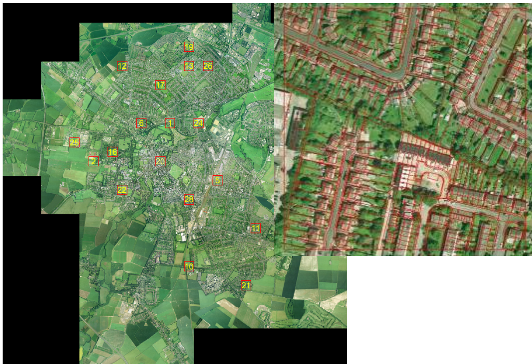
Figure A1.1: Orthophoto mosaic of Cambridge City with the 250 x 250 m 18 sample areas within the city of Cambridge. The example square illustrates the detail of the 1:1250 scale Ordnance Survey Master Map.
