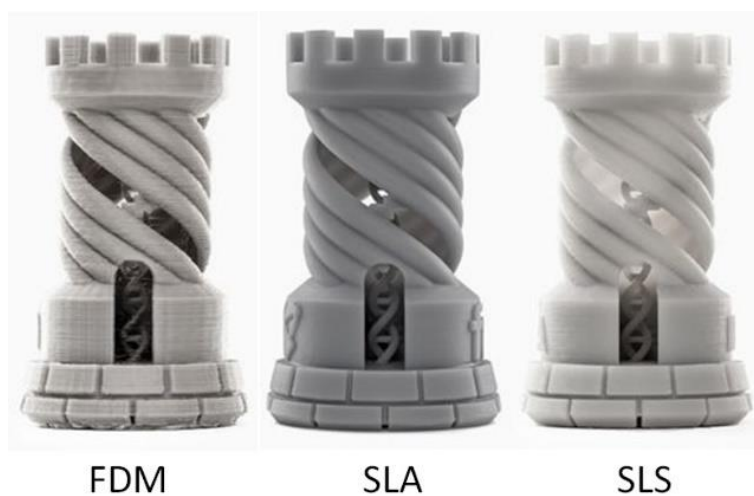
Figure 3-3: Comparative print feature resolution of three additive manufacturing techniques viz., FDM, SLA, SLS [65].
