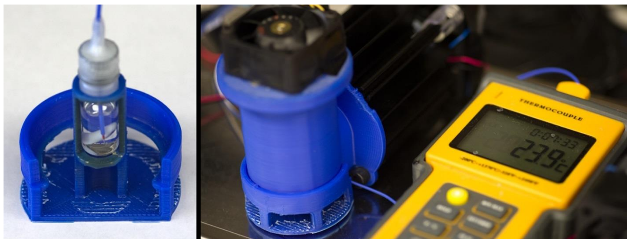
Figure S2.11. Temperature Monitoring Setup. A 0.5 dram vial equipped with a stir bar and 1 mL DMAc was monitored via a type K thermocouple inserted through the septum (left) and sealed with Parafilm. The vial was placed in the photoreactor as shown (right) and irradiated for 3 hours. The photo shown is before irradiation.
