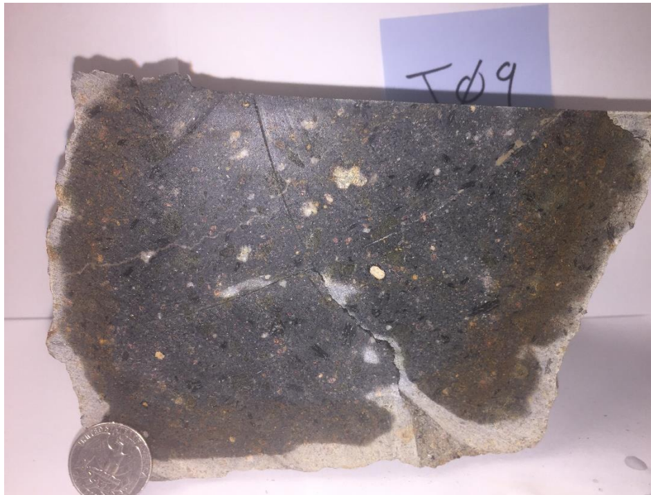
Photograph D3: Lamprophyre J09 in hand sample. Top photo is the natural rock face; the bottom photo is a cut surface sprayed with water to show the macroscopic features of the rock.
