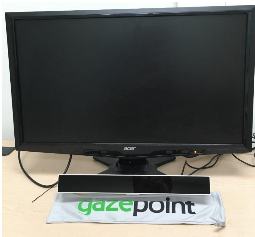
Figure 4 Experiment setup with a Gazepoint GP3 eye-tracker and an Acer monitor
