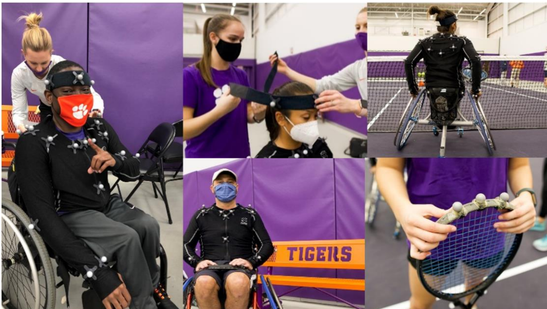
Figure 39. Data collection of wheelchair tennis athletes with reflective markers at desired anatomical locations on the human and segment locations of the racquet and wheelchair.
