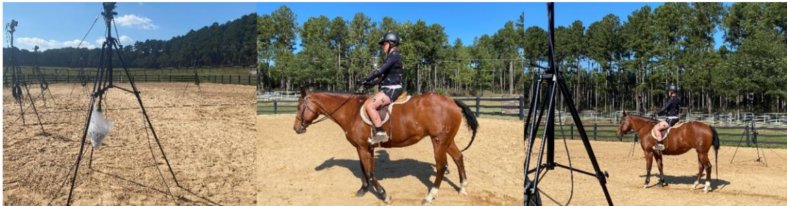
Figure 25. Data collection in outdoor arena with eight motion capture cameras (left) and reflective markers at desired anatomical locations (middle). Horse and rider passed through the motion capture volume to collect kinematic and kinetic data.
