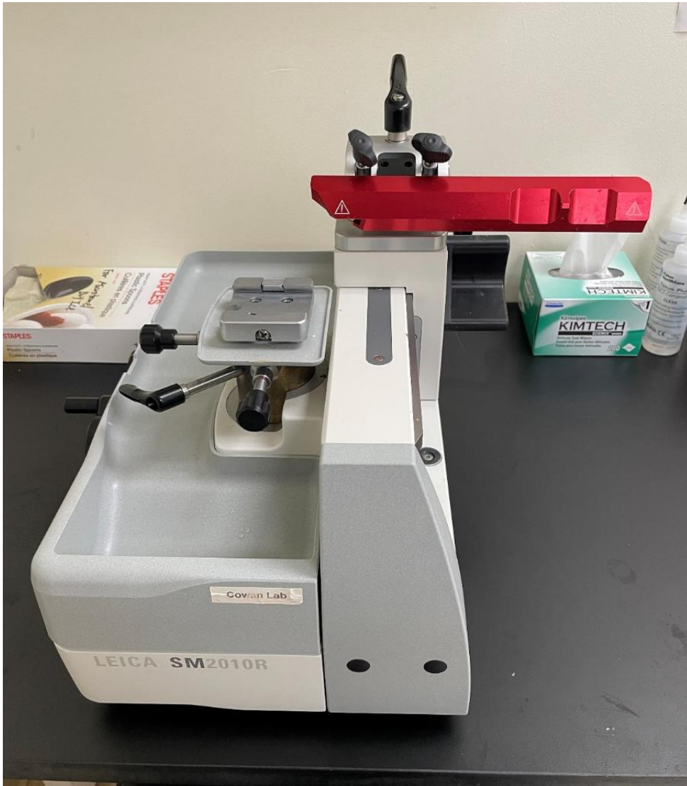
Figure 5.6: Microtome instrument (prior to installing the platform and knife). Photo Credit: Jessica Cooley Coleman.
