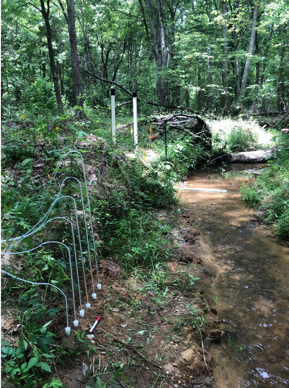
Figure C - 1: Beaver Pond sampling site, with piezometer (left pipe), stream gage (right pipe, protruding into stream channel), and rhizon sippers visible.
