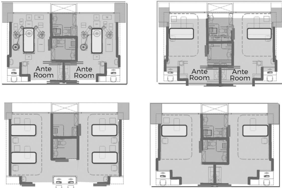
Figure 2.12 the transformation of the NCID inpatient units to expand the capacity and provide isolation capabilities (Soh, 2020)
