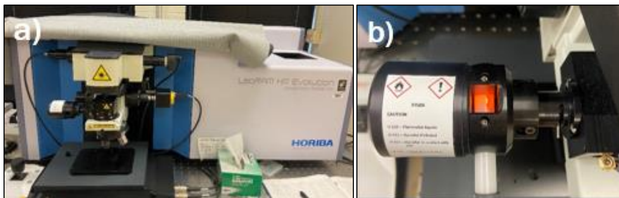
Figure 2.7: a) Raman spectrometer setup with b) neon lamp reference.
