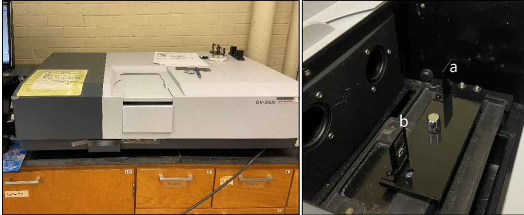
Figure 2.8: UV-Vis Spectrometer (left) and stage (right) with a) reference and b) pair of identical customer-designed sample holders. The sample, a crystal, can be observed on the (b) sample holder.
