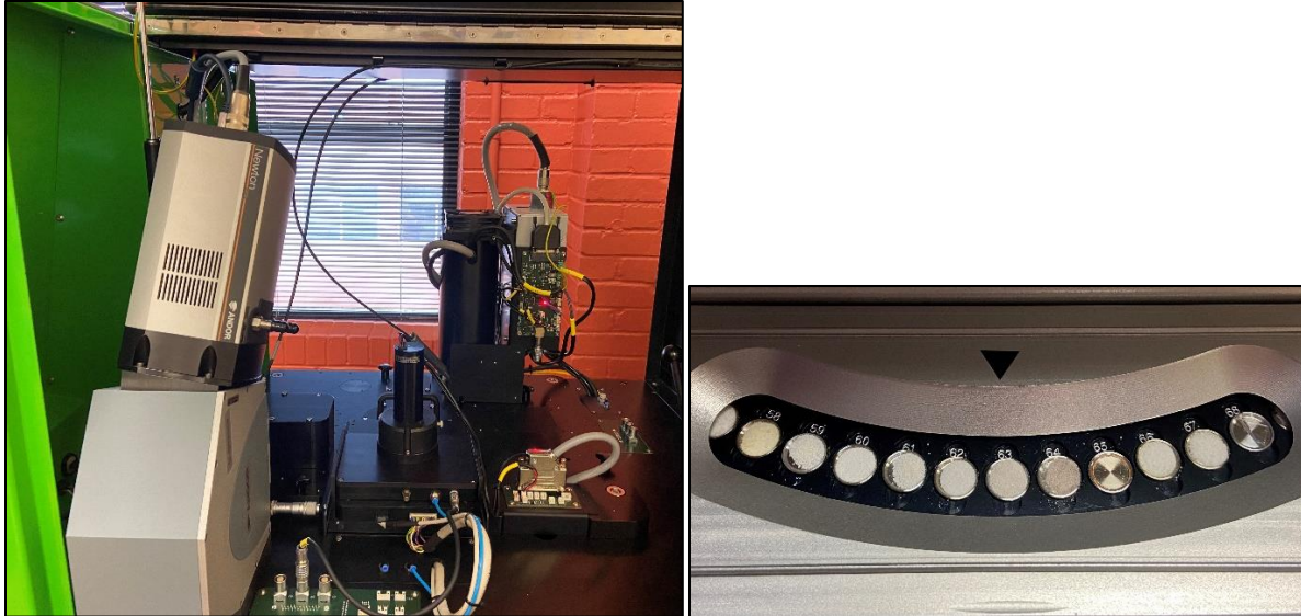
Figure 2.11: Photograph of the Freiburg Instruments Lexsyg spectrofluorometer showing the spectrograph (bottom) coupled to the CCD detector (top), the optical fiber, and the X-ray source in the back. The small cylinder at the center corresponds to the photomultiplier tube. The sample wheel is shown on the right.
