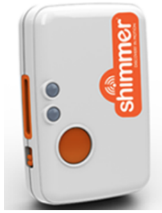
Figure 1.2: A Shimmer3 device for data collection. The device has an orange switch on the side and an orange button for starting the record or ending the record.
