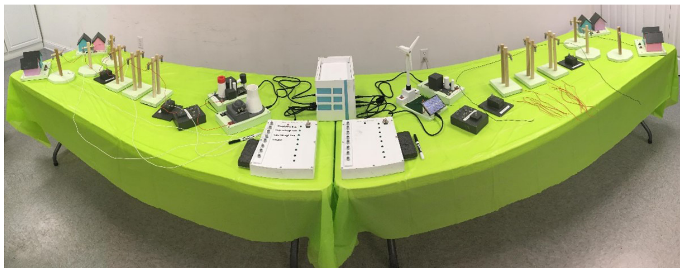
Figure 1. Smart grid for schools kit used for developing hands-on learning activities.
