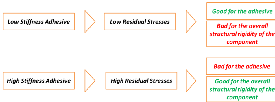
Figure 24. Effect of the choice of adhesive on the adhesive bond and the body structure stiffness
