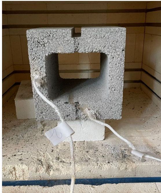
Figure 30 Uniformity Test Setup (results of uniformity tests are shown in Ch. 4)
