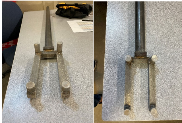
Figure 32 Tool used for extraction of block.
