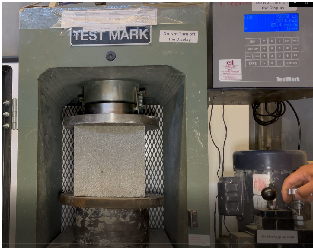
Figure 29 Compressive Testing Machine used for experimental program.
