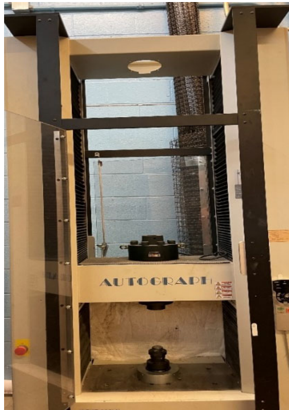
Figure 27 Universal Testing Machine used for Experimental Program.
