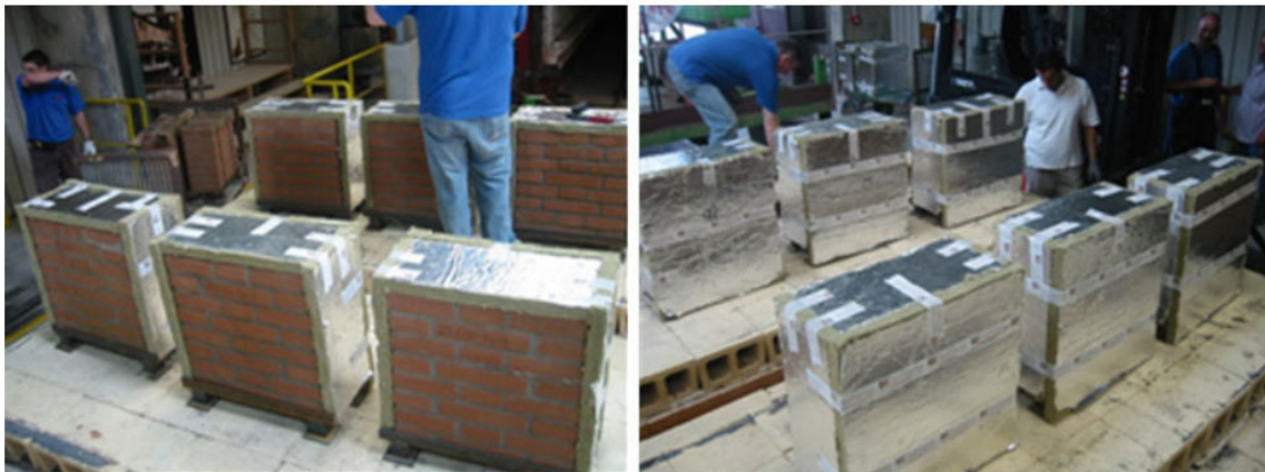
Figure 11 Wallettes specimens to be put to fire tests as per [33]
