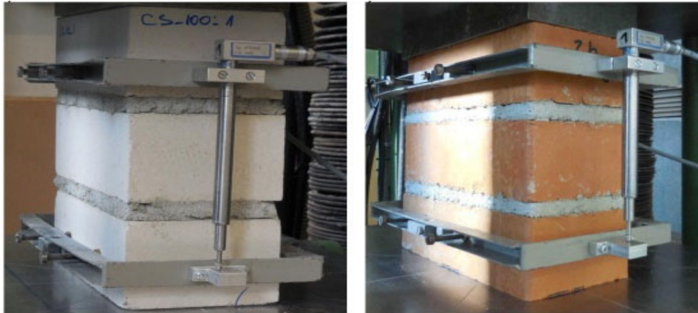
Figure 6 Brick prisms under compression strength test (note: Left – calcium silicate brick prism, right – clay brick prism)
