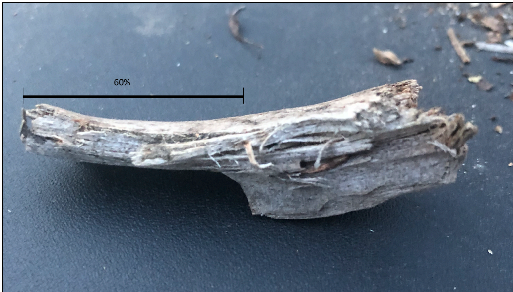
Figure 1.9: Example of measuring guidelines for classifying masticated fuels in destructive sampling for the 1-hr time lag category. With 60% of the woody material measuring below 0.635 cm, this piece of woody material is classified as a 1-hr fuel.
