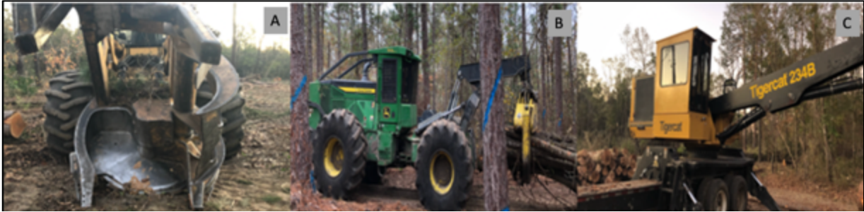
Figure 3.2: Tigercat 720G drive-to-tree feller-buncher (A), John Deere 748-II series, dual-function rubber-tired grapple skidder (B), 234B Tigercat trailer-mounted knuckle-boom grapple loader and pull through delimeter (C) in a Southern pine seed-tree harvest in Camden, SC.
