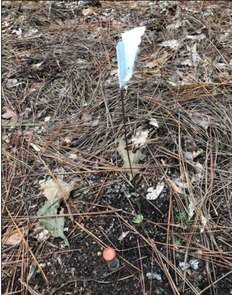
Figure 1.6: Tensiometer (15.24 cm) placement for one sampling point during pre-harvest measurements on Hardscramble in Camden, SC.
