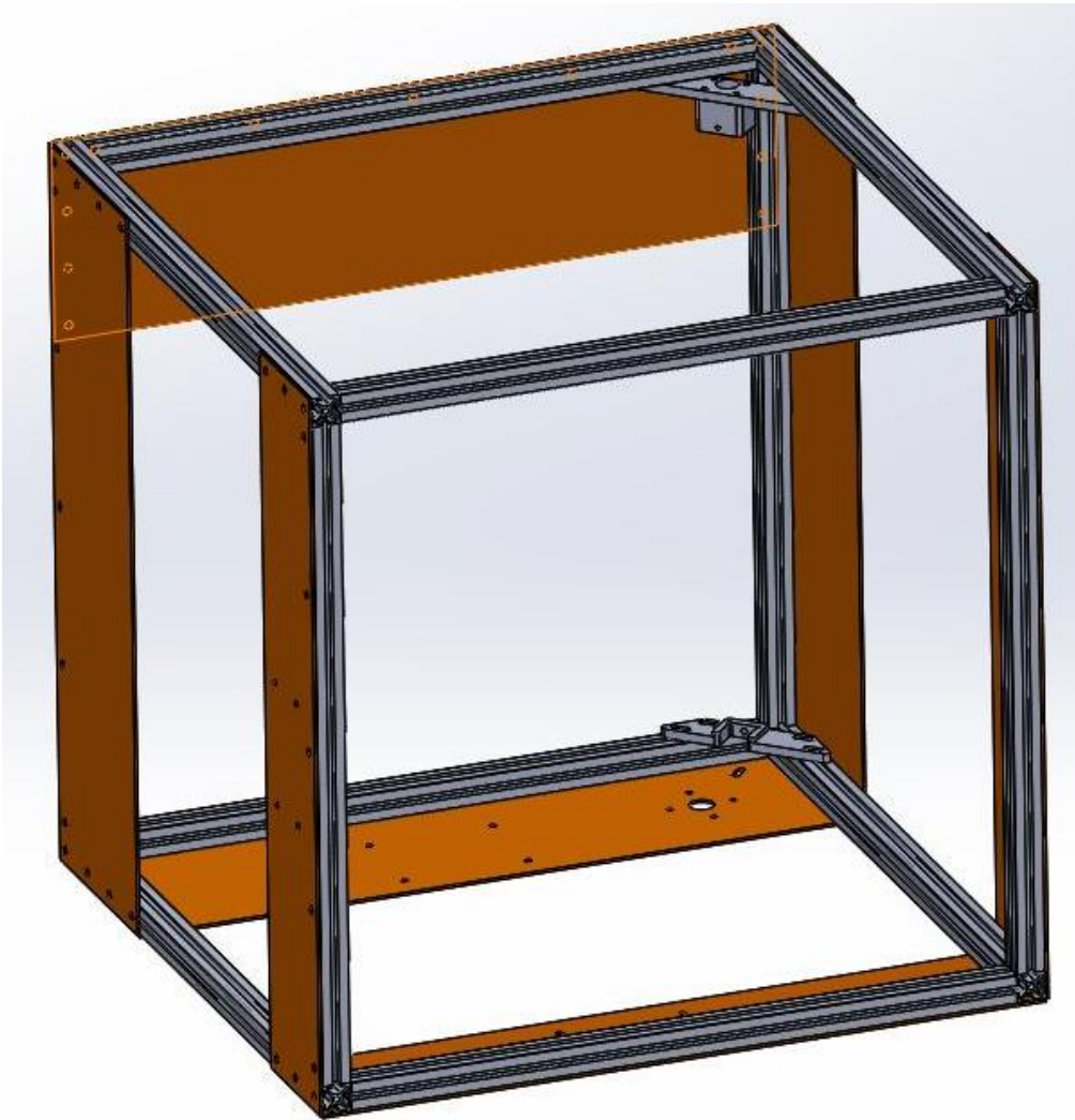
Figure 2.3 3D printer frame consisting of aluminum extrusion and aluminum plates.
