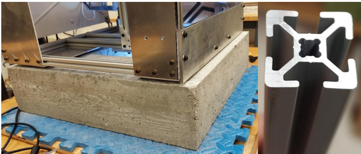
Figure 2.4 (Right) The concrete base used to anchor the 3D printer. This base weighs 105 pounds. (Left) The 20mm x 20mm aluminum extrusion profile used to construct the printer frame.
