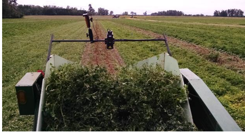
Figure 4.4. 2018 mounting configuration of radar ground speed sensor, center of digger, and high-speed camera, to the left of the radar sensor.
