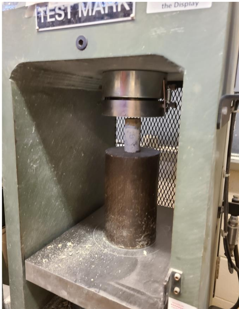
Fig 4.5: Compression test of concrete core
