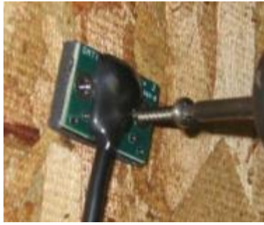
Fig 4.1: Point Moisture Measurement (PMM)
