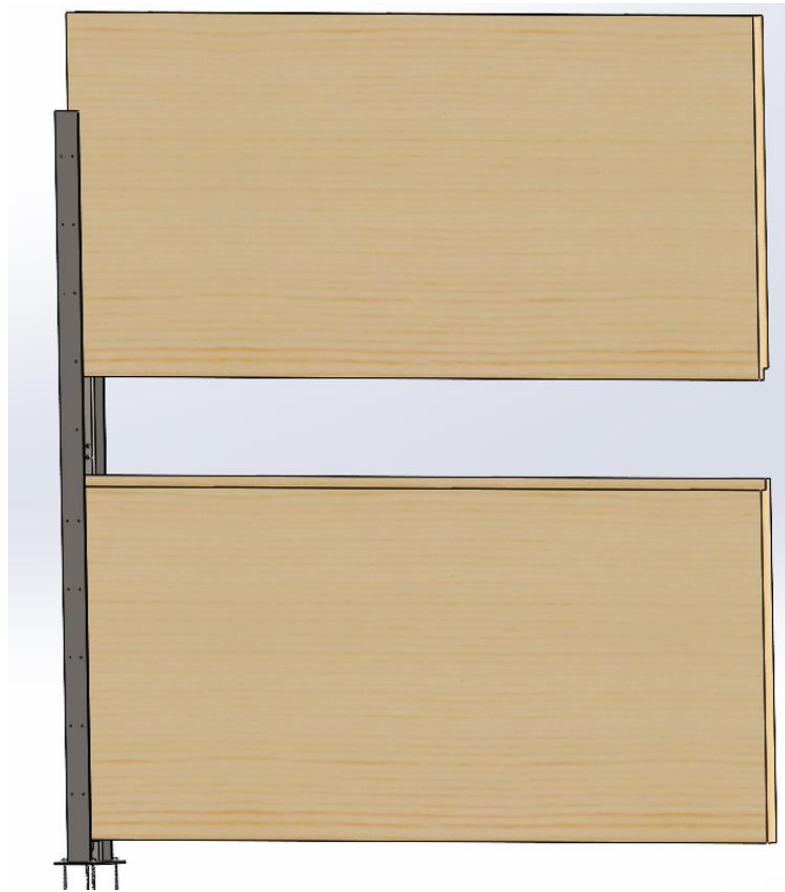
Fig 3.5: Installation of the CLT Panel
