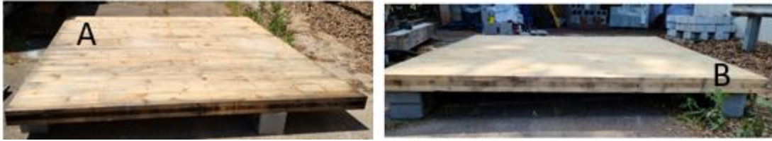
Fig 4.7: Original CLT panel (A), Sanded CLT Panel (B)
