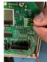
Figure: Twist the green and yellow wires before connecting to the A2/A3 unit.
