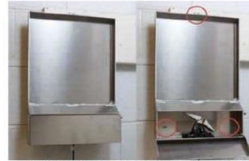
Rain Gauge with cover closed and open. When open, 3 fastening locations are available
