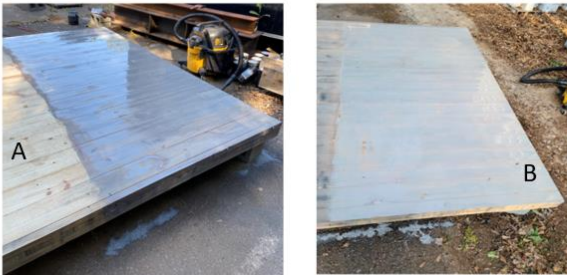
Fig 4.8: First coat of TeakLife coating (A), First coat of WoodForce coating (B)
