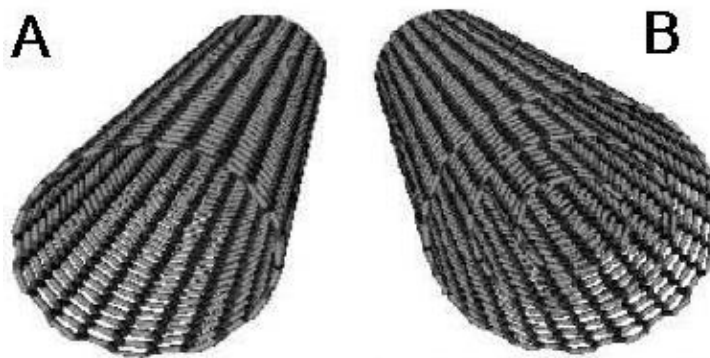
Figure 2.1. 3D image of SWCNT (left) and MWCNT (right) (20)
