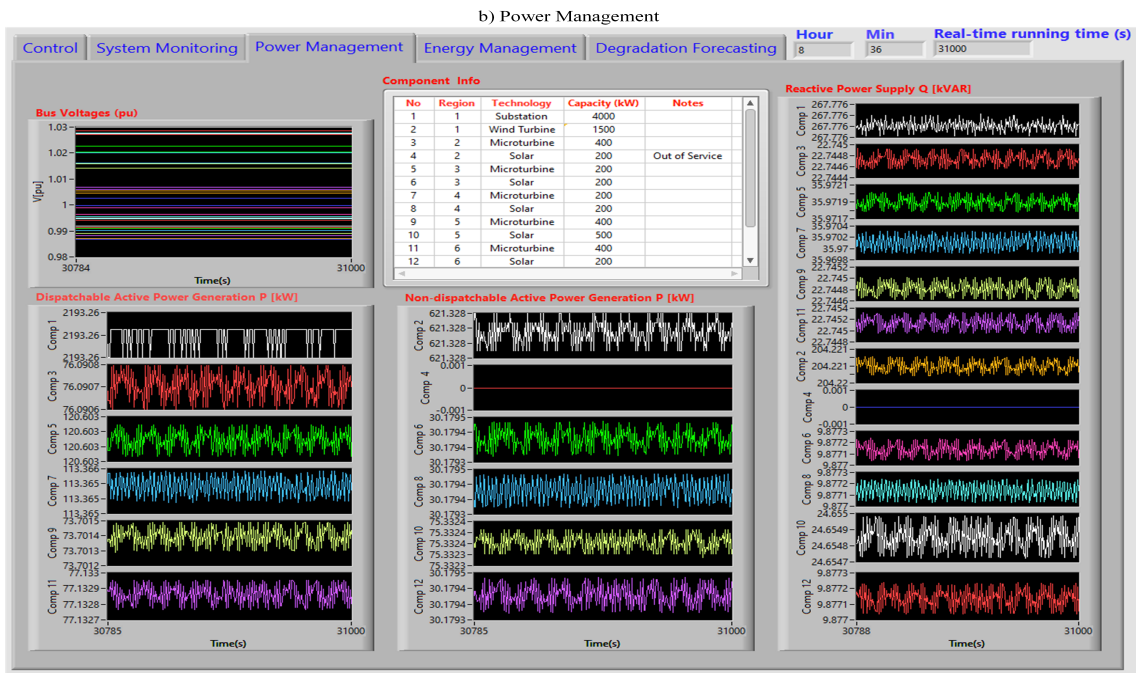
Figure 6.3: HMI display: a) System Monitoring screen b) Power Management screen.
