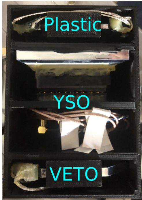
Figure 3.8: Photograph showing the 3D-printed implantation box containing the front plastic detector, YSO implantation detector, and VETO detector.
