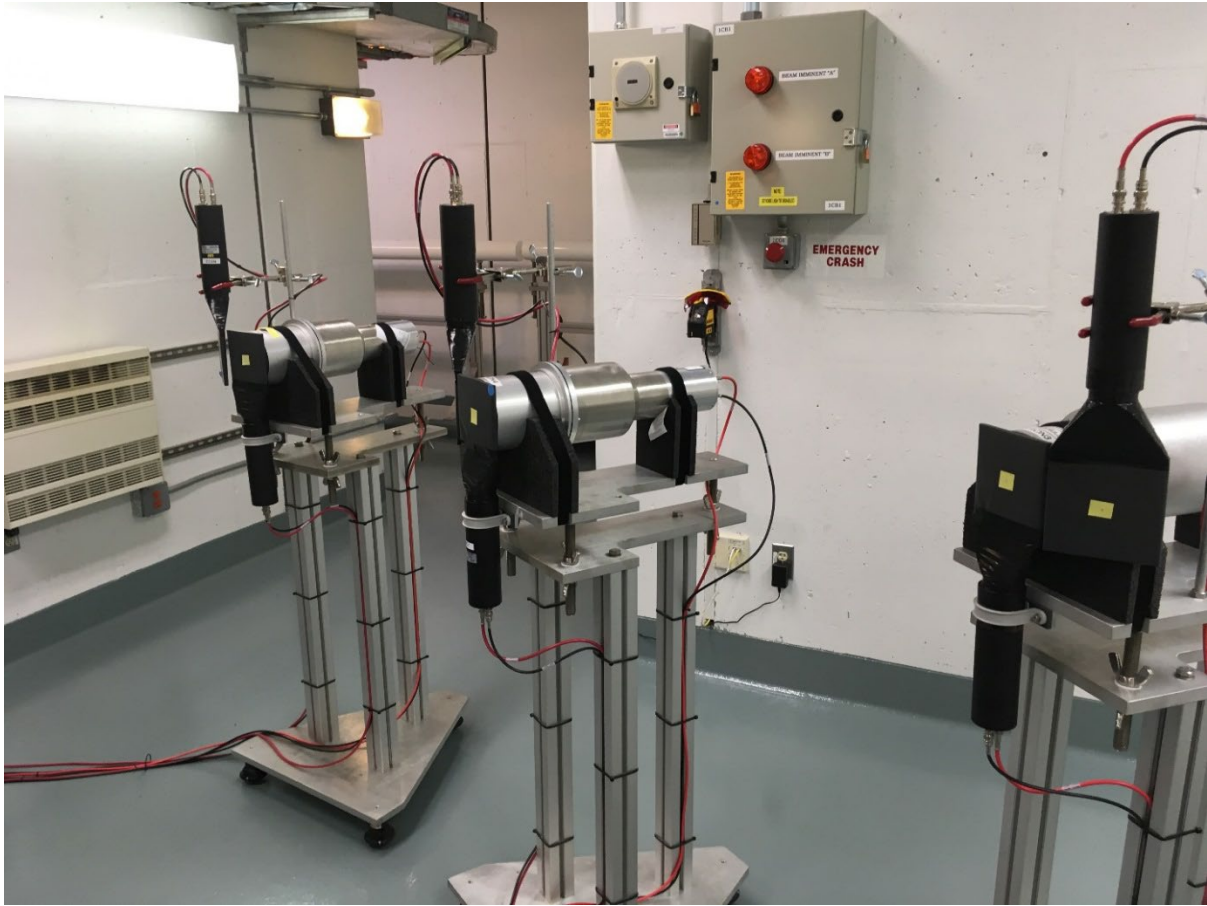
Figure 3. From left to right, the 80°, 60° and 45° liquid scintillator arrays with their accompanying solid plastic detectors. The liquid scintillators are the cylindrical detectors (aluminum housing), and the solid plastic scintillators are the black, 5-inch by 5-inch detectors. As shown in Fig. 2, two sodium iodide (NaI) detector arrays were placed to the right of the beam direction, with the centers of the arrays placed at 10° and 30°. As with the other detectors used in the measurements, the centers of the NaI arrays were placed at beam height. These detectors were used for secondary charged particle detection. Each NaI detector was a 10.16-cm x 10.16-cm x 40.64-cm rectangular block surrounded by a 0.159-cm thick aluminum housing. Each NaI array consisted of two NaI detectors placed side by side, with three solid plastic scintillators placed directly in front of the NaI detector closest to the upstream target. The faces of the plastic scintillators and NaI were oriented perpendicular to the line connecting their centers to the center of the upstream target. The data from the NaI served three purposes: (1) to extend the dynamic range of light charged-particle energies measured at 10° and 30°, (2) to provide finer granularity in the angular distributions of the spectra, and (3) to provide an internal consistency check of the methodologies used in the data analysis, by comparing with similar data from the liquid scintillators at 10° and 30°.
