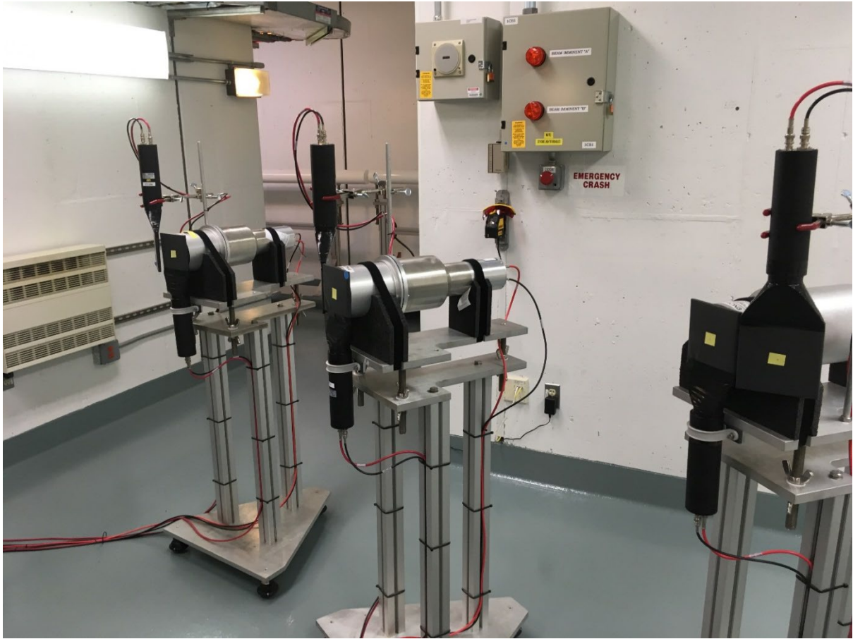
Figure 3. From left to right, the 80°, 60° and 45° liquid scintillator arrays with their accompanying solid plastic detectors. The liquid scintillators are the cylindrical detectors (aluminum housing), and the solid plastic scintillators are the black, 5-inch by 5-inch detectors
