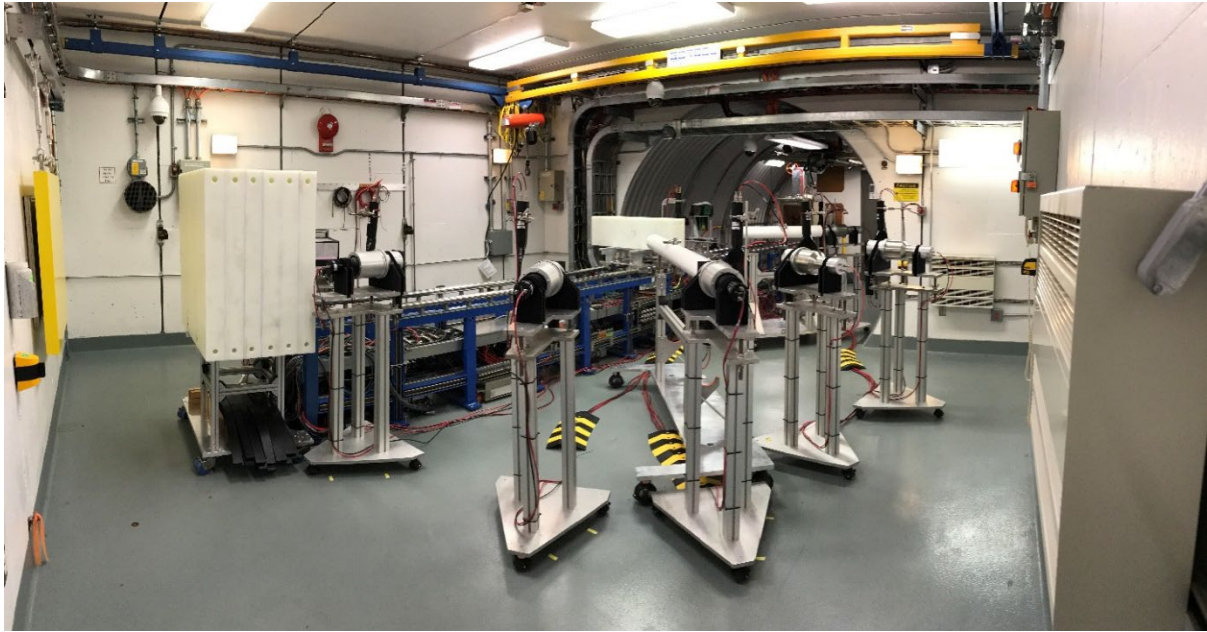
Figure 5. The 2-m and 1-m long shadow bars (white steel cylinders) aligned between the center of the 20 g/cm 2 upstream polyethylene target and the 45° and 135° liquid scintillator detectors.
