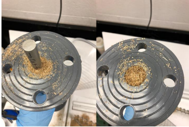
Figure 2-4. Clogging event for lignocellulosic biomass in a bench-scale reactor.
