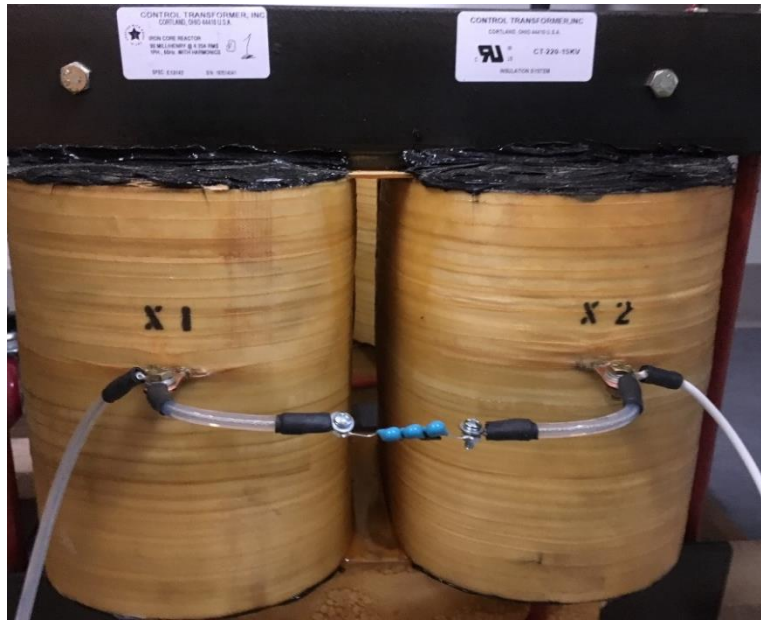
Fig. 4- 4. High voltage load inductor with external capacitor to increase its EPC.
