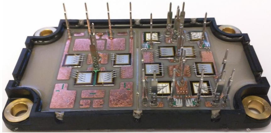
Fig. 4- 13. 10 kV SiC MOSFET module (H-bridge) packaged by Danfoss.
