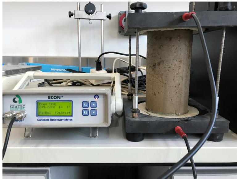
Figure 9: Bulk resistivity test setup
