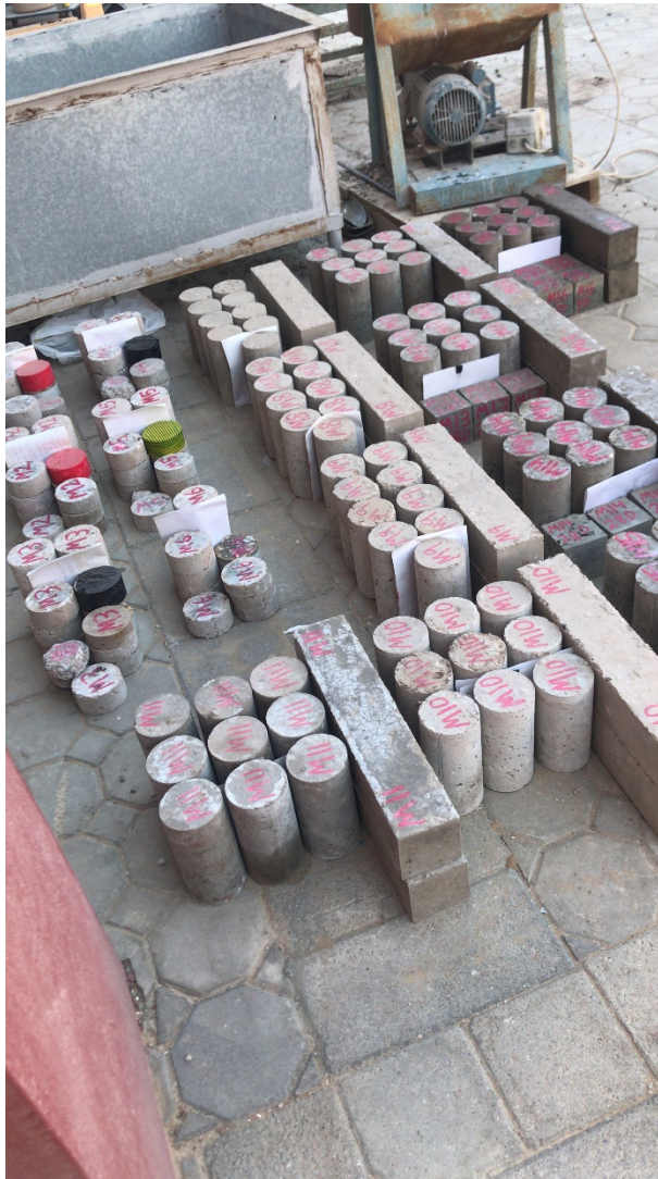
Figure 5: Hardened geopolymer concrete specimens
