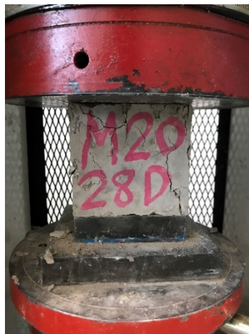
Figure 6: Compressive strength testing of geopolymer concrete cube
