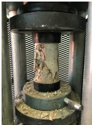
Figure 7: Compressive strength testing of geopolymer concrete cylinder
