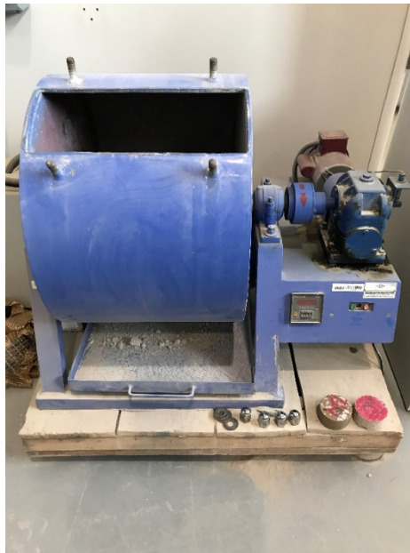
Figure 11: LA abrasion test machine
