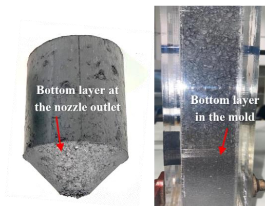
Figure 3.30: Compaction of paste comparison: in a nozzle (left) and manual ramming (right)
