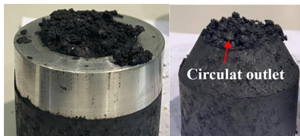
Figure 3.27: Forth trial with 42 mm circular outlet with no extrusion with extrusion load up reaching 25 kN
