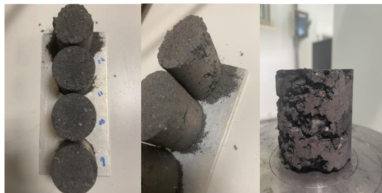
Figure 3.16: Before compression test of 45 kN samples baked at 600°C
