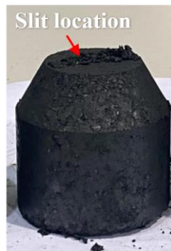
Figure 3.25: Third Trial with no extrusion up to 31 kN with nozzle of an angle of 60° and a slit outlet
