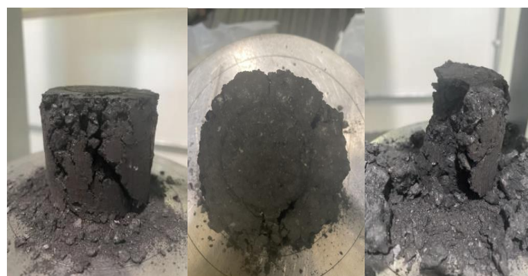
Figure 3.17: After compression test of 45 kN samples baked at 600°C
