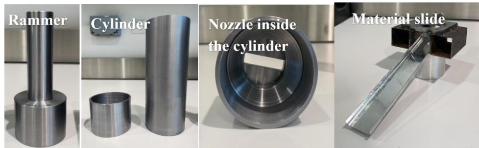
Figure 3.19: Set-up of extrusion experiments
