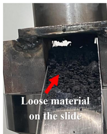
Figure 3.29: Ramming paste at the nozzle exit sliding uncompact
