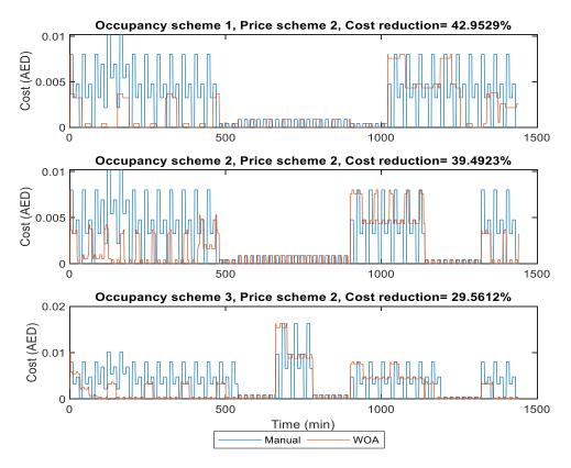
Figure 23: Manual controller cost vs WOA cost for price scheme 2
