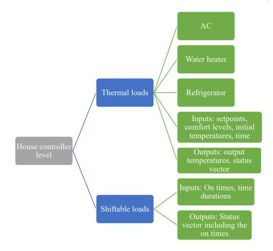
Figure 5: Full house controller model structure
