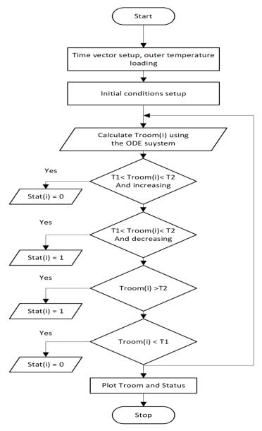
Figure 3: Cooling thermostat system (AC)
