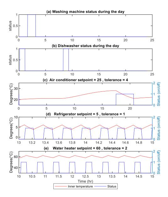
Figure 15: Full house controller output
