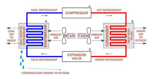
Figure 2: Air conditioner cooling cycle
