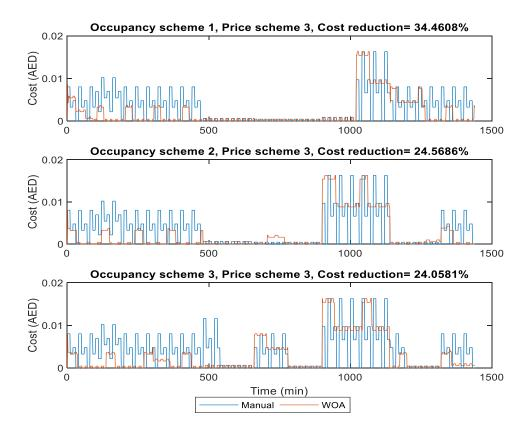
Figure 24: Manual controller cost vs WOA cost for price scheme 3
