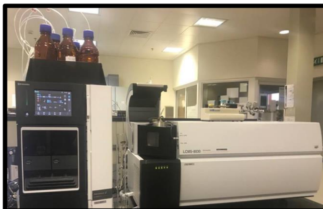
Figure 10: LC-MS/MS used to analyze chiral PCs
