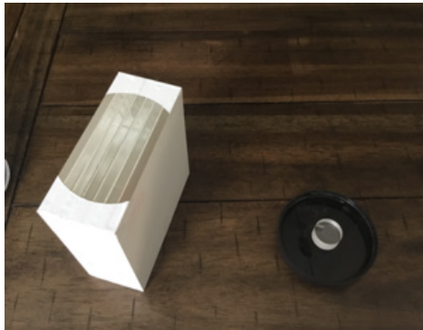
Figure 3. Composite ZEBRA (left) vs. Non-composite (single crystal) Lu 2-x GdxSiO 5 (LGSO). [3]
