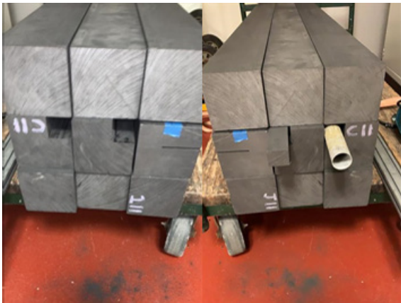
Fig. 5. Examples of unloaded (left) and loaded (right) unit cells (Author picture)
