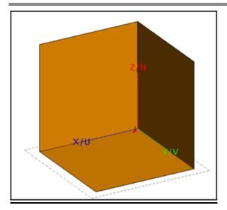
Fig. 2. Corner reflector antenna construction
