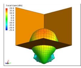
Fig. 3. 3D Radiation Pattern of Corner Reflector Antenna
