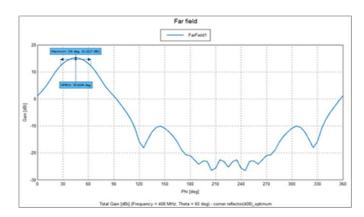
Fig. 10. Half power beam width (HPBW)
