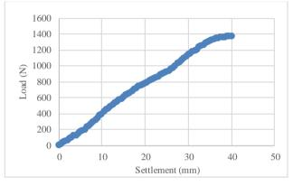
Figure 3: Load settlement curve without stone column
