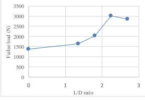
Figure 9: Failure load at different L/D ratio
