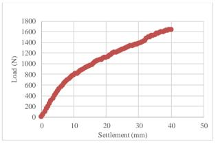
Figure 4: Load settlement curve stone column 135mm length
