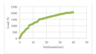
Figure 5: Load settlement curve stone column 180mm length
