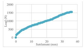
Figure 7: Load settlement curve stone column 270mm length
