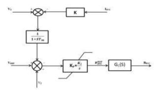
Fig.1. Model of svc controller
