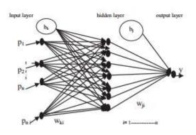
Fig.3. Architecture of multi-layer-nfeed forward ANN
