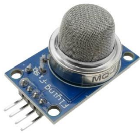
Gambar 3. Sensor Gas MQ-02 (Sumber : www.arduino.cc )
