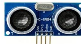
Gambar 2. Sensor Ultrasonic HC-SR04 (Sumber : www.arduino.cc )
